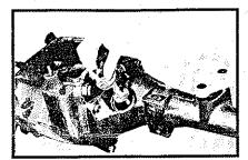
The speedo gear comes out next. The clever swap-meet tape "protecting" the end of the speedo adapter hid stripped-off threads where the cable hooks. No biggie: Common slush-box speedo adapters interchange.
