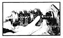
11 Moving on to the tailshaft, remove the gearset and mainshaft after releasing the retaining ring at the front of the extension.
