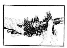
16 The gears and synchros were cleaned, lubed with gear oil, and reloaded on the mainshaft. Make sure that the lugs or slots in the stop rings line up with the struts on the synchrohub so they seat properly.
