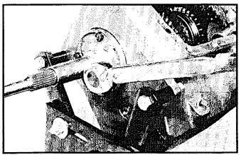
A new seal is installed in the front bearing retainer and lubed (lip to the tranny side), the snap-ring is installed on the bearing, and the retainer torqued in place. Use sealant on the bolts to keep oil from drooling out.
