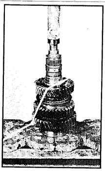
17 With all of the components loaded to the back of the main-shaft, the new bearing is pressed on (outer snap-ring groove forward with the large PN 308 bearing). To keep the gears from sliding back with the shaft upright, the assembly was temporarily tied back with nylon ties and then loaded into the press. Make sure the press platform supports the bearing at the inner race since pressing the bearings by loading the outer race will trash 'em.
