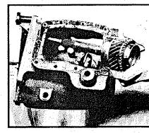
**9** With the countergears sitting on the bottom of the case, remove the bearing retainer and snap ring, then slide out the pinion. Now reach in and lift out the countergears.
