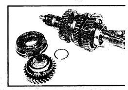
12 Unloading the gears from the mainshaft is a matter of pulling snap rings and sliding the gears off. At the front, the Third-to-Fourth synchro and Third-speed gear come off. At the rear, the bearing is pressed off, followed by First gear, the First-to-Second synchro, and then Second gear. Make sure you keep track of the order of the parts, or have a detailed service manual handy.
