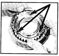
15 To begin reassembly, we cleaned up and reassembled the synchros. Make sure the inner hub is facing the right way and is matched to the correct outer sleeve. Lay the synchro hub on top of a stop ring to hold the parts in alignment, load in the three synchro struts (arrows), and wind in the front and rear springs, centering on two different struts. The new stop rings go in as the gears are loaded on the shaft.
