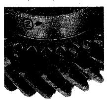
should be sharp, as shown, with a small amount of rounding being generally okay. If you are wondering what contagious disease this gear is afflicted with, it's a brand new gear, coated with Cosmolene. Arrow #2 indicates the actual brake drum area of the gear. This surface should be smooth and free from scoring, galling, or grooves.
