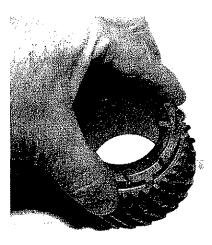
Synchro stop-rings (brass rings) can actually be tested. All that's required is applying a light downward pressure while twisting the ring. With little more than a light press, the ring should seize onto the gear. If this fails, try a new stop ring. Still ng? Time to hunt up a new gear. Apply this test to all 4 speeds, but expect to see the majority of trouble on 2nd and 3rd gears. Like, how often do you power-shift First?
