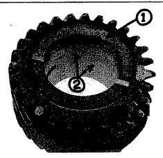
As with the countershaft gear, main gears can sometimes show wear on the thrust (1) and interior bearing surfaces (2), in addition to cone and dog-tooth wear shown in the first photo in "Synch or Swim." Check these carefully for excessive play on your mainshaft. Note that Hemi gears have Oilite bushings on the inside.
