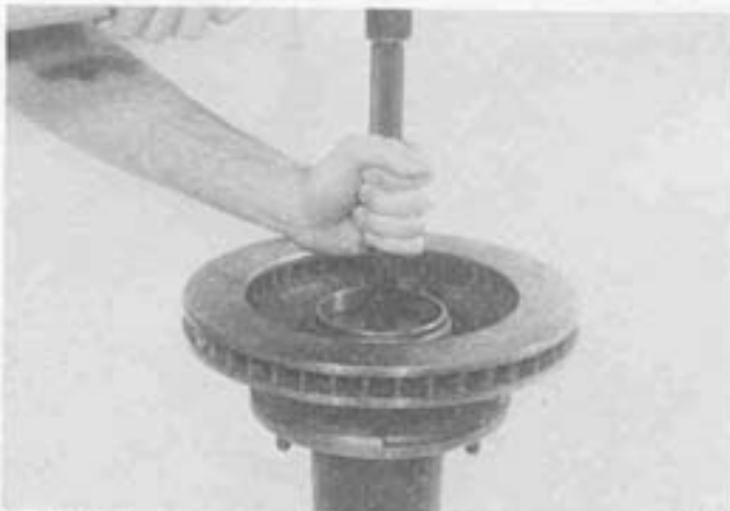
Figure 50 1019-50 Assemble inner wheel bearing cup. Tools: #D-256 Installer, #C-4171 Handle.
